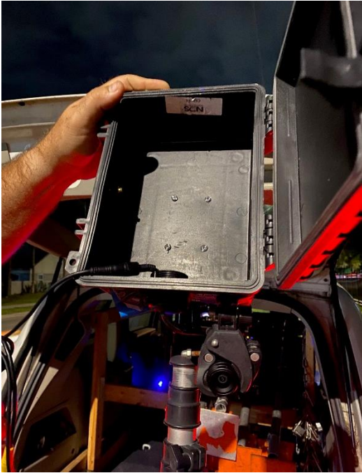
Camera beneath box housing battery and recording device
