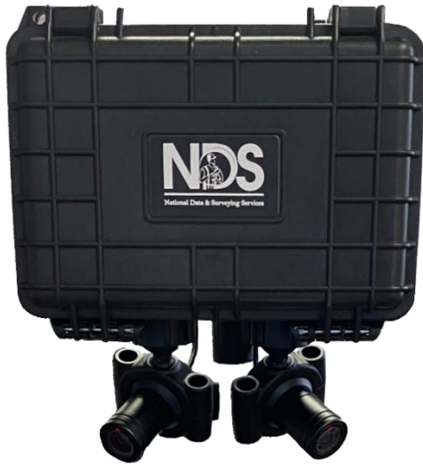
Figure 3. Weatherproof box held battery and recording device
