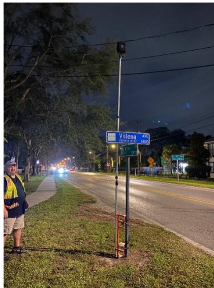
Figure 2. Camera deployed in its telescoped position
