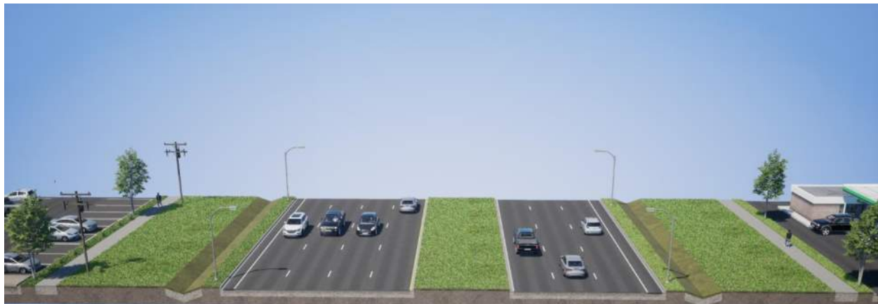
Figure 6: Causeway Boulevard/W. Lumsden Road, Existing Typical Section
