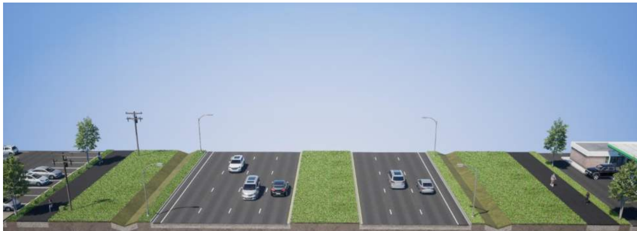
Figure 7: Causeway Boulevard/W. Lumsden Road, Proposed Typical Section
