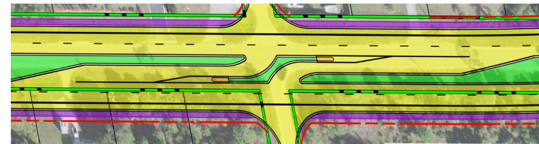
Example Directional Median Opening
