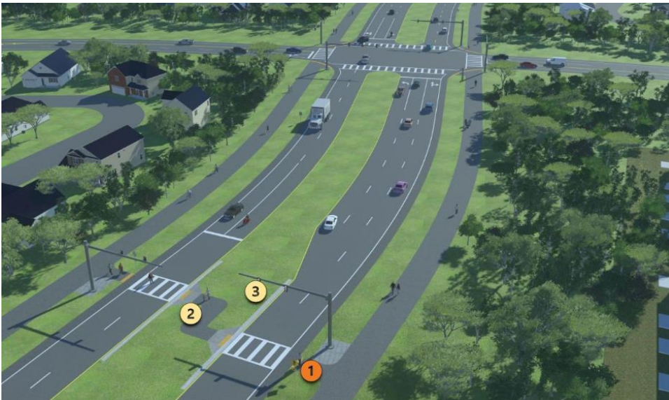
Example 4: 1 – Full stop pedestrian signal. 2 – Refuge island. 3 – Midblock crossing. (Source: Florida Department of Transportation Complete Streets Explorer Tool, flcompletestreets.com .)
